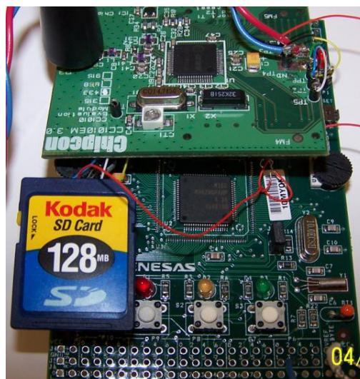
Figure 3. The Renesas M16C 16-bit MCU, Co-S platform, integrated with the Chipcon RISE platform and sporting an SD-Card
